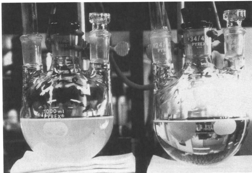
Figure 5. Photograph of reactor vessels blank (left) vs orthoborate treated (right), after standing overnight.
